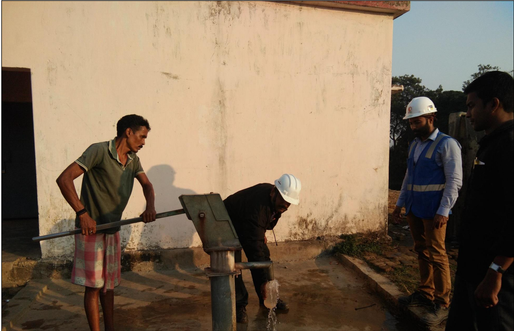
Photograph showing collection of ground water sample from bore well
