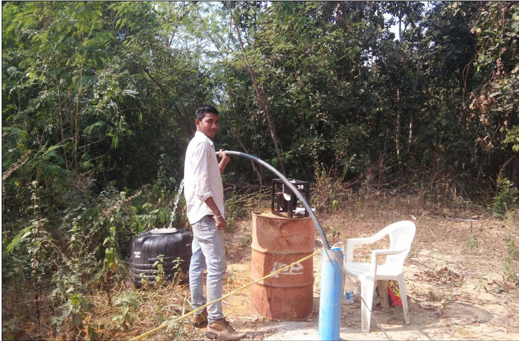
Photograph showing measurement of discharge of bore well during pumping test.
