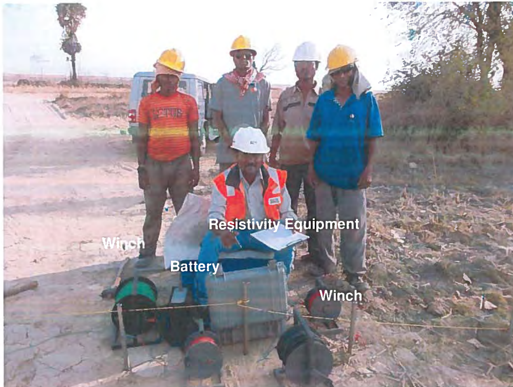
PLATE 4: ELECTRICAL RESISTIVITY SURVEY (SCHLUMBERGER METHOD) WAS CONDUCTED ASH POND AREA
