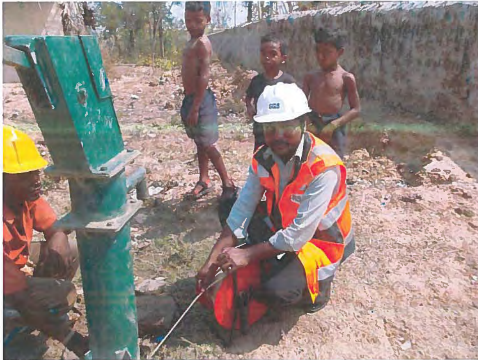
PLATE 3: ELECTRICAL WELL SOUNDER FOR GROUND WATER LEVEL MEASUREMENT
