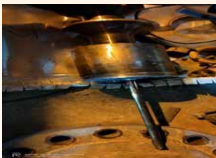
CEP-4B RC valve stem bend and plug profile damaged
