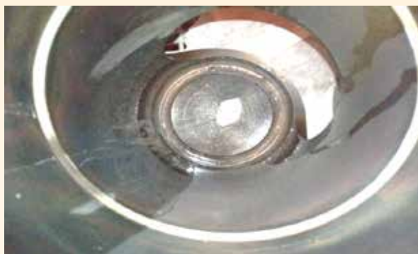
Seat Ring Damaged-HWL CV-2
