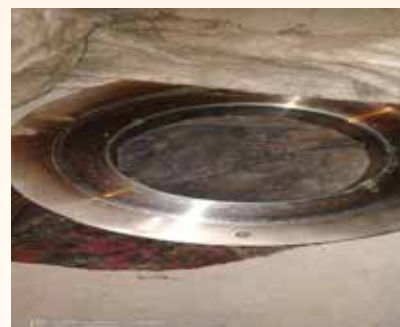
CEP- RC valve sheet after machining
