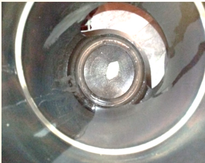
Seat Ring Damaged-HWL CV-2
