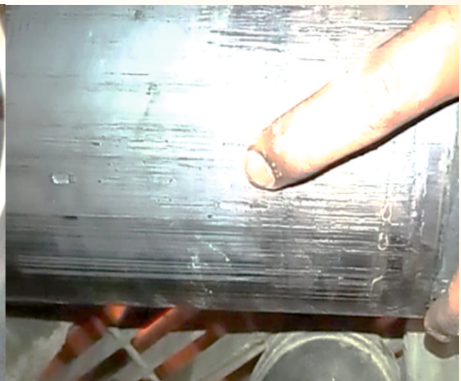
(Scoring marks observed in plug of HWL)
