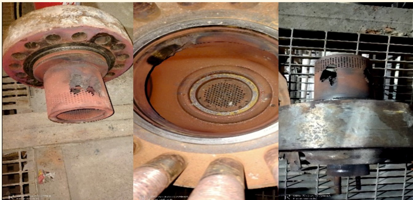
(BEFORE) Damaged TDBFP-4A & 4B Internals & body
